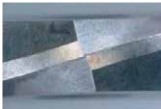
加工1,248分钟后的刀尖状态 Cutting edge after 1,248 minutes of milling.
