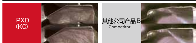
【FCD600】加工1,600孔时的磨损比较 Wear comparison after 1,600 holes of drilling
