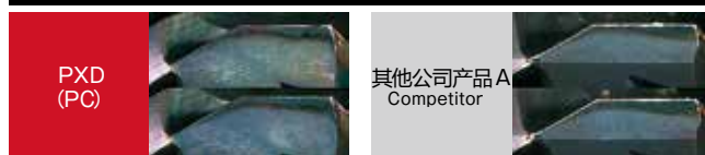
加工900孔时的磨损比较 Wear comparison after 900 holes of drilling
