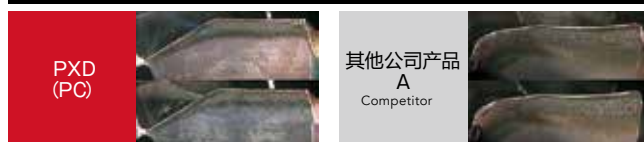
加工1,000孔时的磨损比较 Wear comparison after 1,000 holes of drilling
