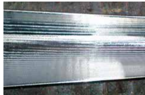
加工1,248分钟后的刀尖状态 Cutting edge after 1,248 minutes of milling.
