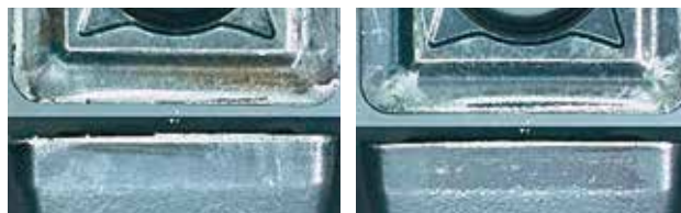
刀片磨损情况的照片(加工5个孔时) Photo of insert wear width (after 5 holes)
